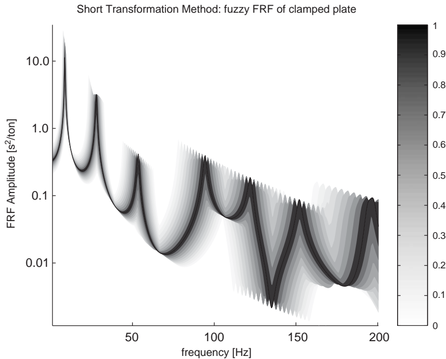
Fig. 14. Fuzzy FRF of the clamped plate in Fig. 12, obtained with the Short Transformation Method in the range 0–200 Hz. A darker colour represents a higher level of membership of the fuzzy FRF output.
